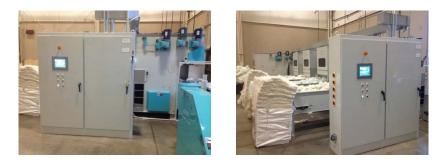
The CCS *UltraLoft* weight control system is a PLC based touch screen system that is manufactured with UL/CE compliant off the shelf components such as Siemens, Allen-Bradley and others. The *UltraLoft* system includes recipe management, active weigh control, trending, reporting, help screens, remote support and multilingual text.
