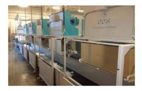
CCS *UltraLoft* high speed openers are manufactured in many different styles; the standard openers are horizontally or vertically fed. The openers can be configured with metallic wire wound cylinders, fully lagged cylinders and claw tooth cylinders depending on the application. CCS *UltraLoft* Blending and Opening systems are capable of producing as much as 1,500 to 2,500 kilos per hour depending on the fiber type, denier, staple length and blend percentages.
